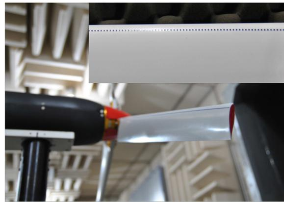
Fig. 10. Small-scale blade and trip strip on the blade surface.
